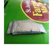
had come loose and was dragging on the track only being held in place on one corner. The violent movement of the metal swinging under the car under high speed at the ½ mile speedway was definitely the issue and Billy did a great job in judging the impact to the handling of the car to bring it home with the first top-10 of the season.
